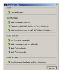
When the tests are complete, the Running Tests dialog box automatically closes, and Admin Center displays the test results in the Connectivity Testing dialog box.
