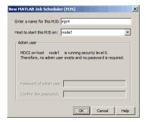
Alternative methods for starting an MJS include selecting the pull-down MJS > Start, or right-clicking a listed host and selecting, Start MJS.
