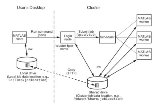
In this type of configuration, job data is copied from the client host running a Windows operating system to a host on the cluster (cluster login node) running a UNIX® operating system. From the cluster login node, the LSF bsub command submits the job to the scheduler. When the job finishes, its output is copied back to the client host.
