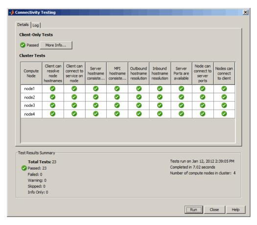
If any of the connectivity tests fail, double-click the icon that indicates a failure to get information about that specific test; or use the **Log** tab to get all test results. With this information, you can refer to "Troubleshoot Common Problems" on page 2-22. If you need further help, contact the MathWorks install support team.
