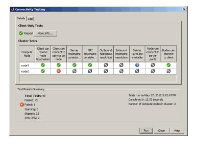
Double-click any of the symbols in the test results to drill down for more detail. Use the **Log** tab to see the raw data from the tests.
