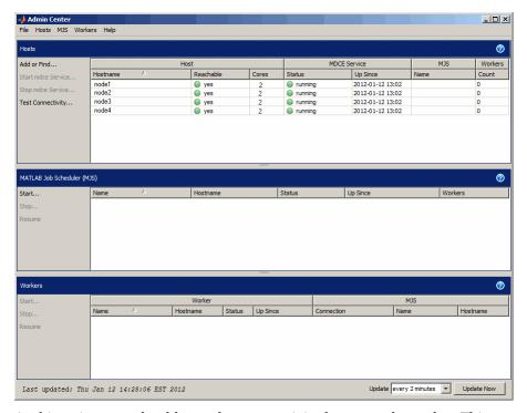
**e** At this point, you should test the connectivity between the nodes. This assures that your cluster can perform the necessary communications for running other MATLAB Distributed Computing Server processes.
